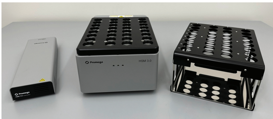
Figure 1. Power Supply, HSM 3.0 Instrument and Tube Rack on Tube Rack Stand (from left to right).
