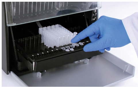
Figure 48. Closing the elution tube caps.
