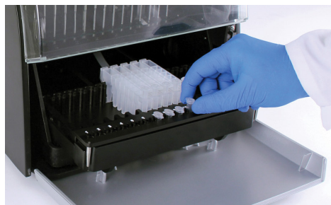
Figure 49. Removing the elution tubes and the deck tray.
