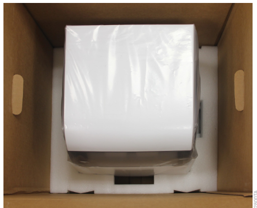
Figure 62. Maxwell® CSC Instrument in correct orientation in the box.
