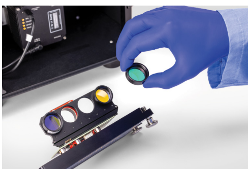
Figure 18. Panel A. Removing the front panel. Panel B. Filter slide panel. Panel C. Removing emission filters.
