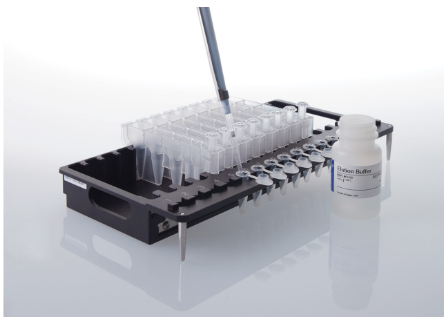
Figure 3. Setup and configuration of the deck tray(s). Elution Buffer (RCFD) is added to the elution tubes as indicated. Plungers are in position #6 of the cartridge. Deck tray shown is from the Maxwell® CSC Instrument (Cat.# AS6000).
