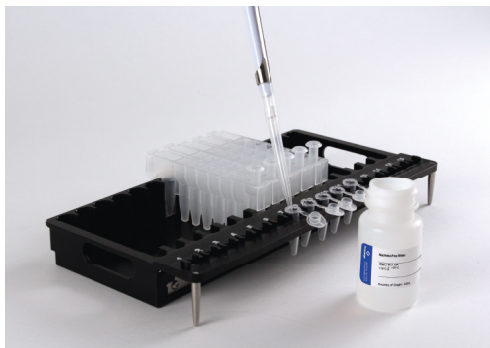
Figure 1. Setup and configuration of the deck tray. Nuclease-Free Water is added to the Elution Tubes as indicated. Open Elution Tubes before beginning an extraction method.
