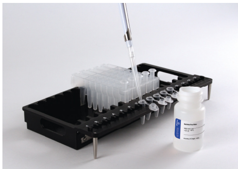
Figure 7. Setup and configuration of the deck tray. Nuclease-Free Water is added to the Elution Tubes as indicated. Open Elution Tubes before beginning the extraction method.
